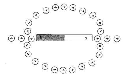
The field can then be drawn using magnetic field lines, in much the same way that we draw electric fields.
