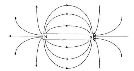
Another way to visualize magnetic field lines is by placing a sheet of paper over a magnet, or magnets, and sprinkling iron filings on the paper. The filings will arrange themselves along the magnetic field lines, thus revealing the pattern.
